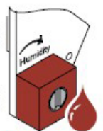
Fig. 6 Humidity regulator Humidity 60-95 %
